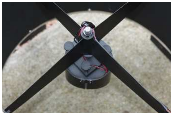
Picture 6: Adjustment screws on the secondary mirror. While in a mono-telescope these are used to collimate the secondary mirror, with a binoscope they are used to re-collimate the primary mirrors!
