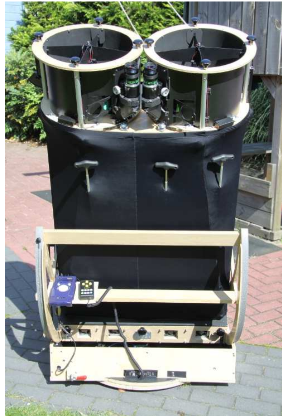
Picture 4: The grips of the aluminium collimation rods are placed at shoulder height of the observer.
