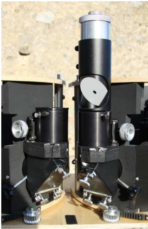
Picture 7: Like Picture 5, but now the Howie Glatter tuBLUG ( http://www.collimator.com//tublug.htm ) is placed between the single beam laser and the focuser/ diagonal. In this way, re-collimation of the primary mirrors can be followed with ease.
