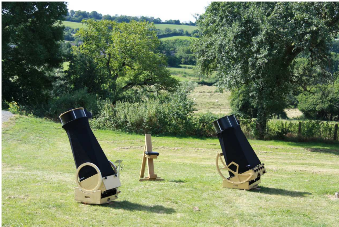
Figure 1. At the left my 16 inch f/4.5 mono-Dobsonian telescope and at the right the 2 x 13 inch f/5.0 binoscope. For more pictures of these instruments see my website ( http://arieotte-binoscopes.nl/Binoscopes.htm )
